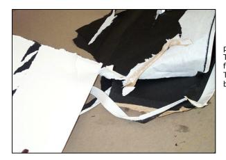
photo 2 The pressure-sensitive Velcro and linen tapes used to help seal the filler boards to the metal frame edges was still extremely aggressive. The linen carrier had dried out and the adhesive had peeled from it, but the saturation and bond remained aggressive to the paper and metal.
