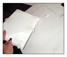
Looking further into the frame there was no detectable visible damage or chemical reaction to the hot glue. The lasting bond of the 3M #3797 neutral pH hot glue stood solid. Though the nature of hot glue permanence may be generally frowned upon for use in a frame, there are situations where it may be applied with no damage. This traveling floated cast paper image makes a good case for that.
