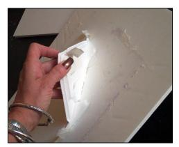
photo 3 Hot glue was used to bond the float panel to the backing and was inseparable, massive Tpeel strength.
