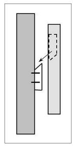
diagram 1 Wood Cleat Top bar is mounted inside box with bevel cut bottom. Mount piece is narrow enough to fit inside the box is mounted to the wall.
