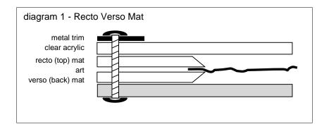
The presentation unit is held together with strips of black metal surrounding the perimeter of the face of the art using short screw bolts to snuggly hold it together. All screws and metal trim on the front were painted black **(photo 2)**. The detail of the screws at the back corner of the frame show they were perfectly sized to fit the thickness of the package.
