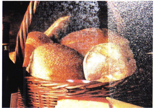
The surface finish (left) appears mottled or scuffed when the sponge is not used. A correctly mounted finish (right) reflects the texture of the sponge.
