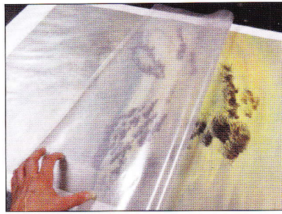
Cut the laminate larger than the poster, peel back the film, align the poster between laminate and liner, and close the vinyl film over the print.
