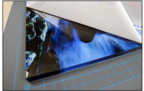
photo 4 Remove the release film from the front of the acrylic and check carefully. Once checked be very careful not to damage the surface so reapplying the protective sheet is suggested.
