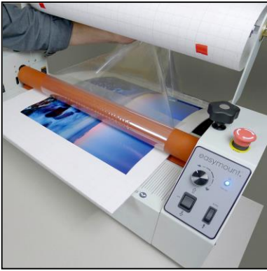
photo 3 Pass the print through the RL in one smooth motion removing the release liner film as it advances through the rollers. Film will be mounted to the surface of the print with the release film still on the top surface.
