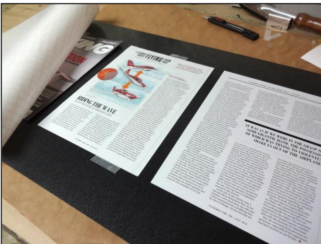
photo 4 After preliminary alignment the pages were temporarily held in place top and bottom with a small piece of low tack 3M 811 removable tape.
