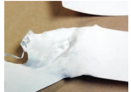
TerraSkin recoils badly at highest setting of a clothes iron but is fine with tacking iron. Heat should remain below 150oF. TerraSkin UV degradable paper is marketed as "paper made of stone."
