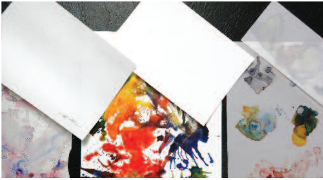
(L-R) TerraSkin made of calcium carbonate/polyethylene resin; Yupo polypropylene opaque white 74# and 144#; and Yupo translucent 104#.
