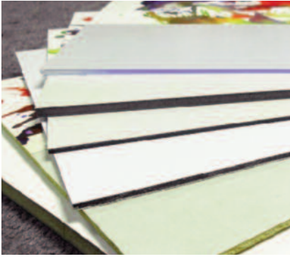
Neschen gudy 831 was pre-mounted to hardboard; ACM; 6mm Black Sintra, 1/4" Black Gator; and 1/8" clear acrylic then half was mounted with 74# Yupo using a Drytac JetMounter roller. Left half was then mounted with painted Yupo tester to coated board using same roller.
