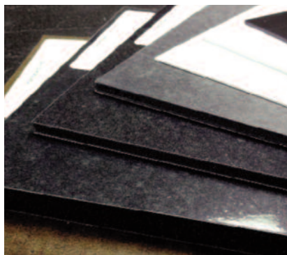
(clockwise- bottom to top) \frac{1}{8} " hardboard; Coda Cold-Mount Black \frac{1}{2} "; \frac{1}{4} " Gatorboard with back coating to counter warping; \frac{1}{4} " Black Gator (no backing); Sintra 3mm, 6mm, and 3mm black.
