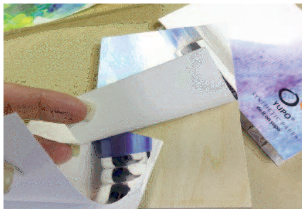
Preliminary wet and spray adhesive tests (clockwise from top). Spray peels from hardboard; gel on EagleCell is well bonded but shows slight honeycomb; gel on half of a ½” birch panel bonds well; gel on Sintra easily pulls off.
