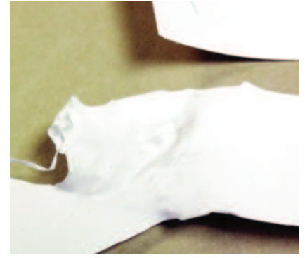
TerraSkin recoils badly at highest setting of a clothes iron but is fine with tacking iron. Heat should remain below 150F. TerraSkin UV degradable paper marketed as "paper made of stone."
