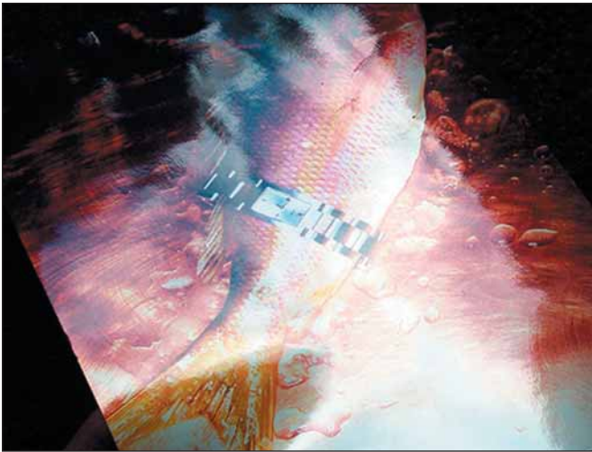
The metallic appearance of the Endura Metallic paper is the result of mica in the paper coating beneath the image.
