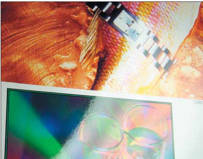
An Océ Lightjet print on Endura Metallic VC (bottom) and an original Kodak Endura Metallic (top). There is a natural orange peel inherent in the Endura Metallic VC paper that was not in the original RC photo paper.
