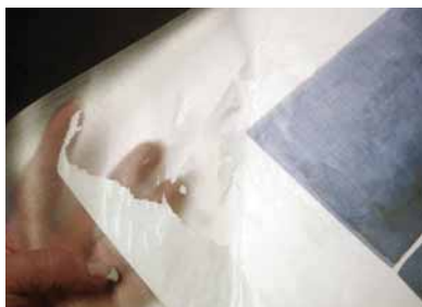
Dry toner was lifted from this print when the laminate was repositioned.
