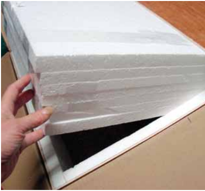
Photo 4: The cardboard box is lined on all sides, top and bottom with 1/4" plywood, and stacked full of sheets of 1" polystyrene making a very rigid package.
