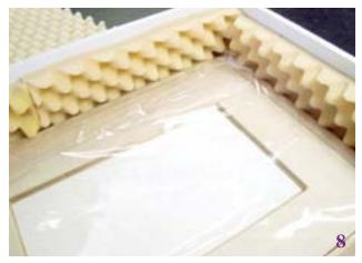
Foam center board has a cushion and is more forgiving than other rigid materials, making it the best choice for a shipping box. This  $\frac{1}{2}$ -inch box has been lined with  $\frac{2}{2}$ -inch eggcrate foam.
