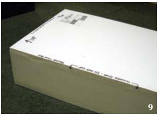
The sealed hinged box is ready to ship. It has been taped with 2-inch-wide heavy duty packing tape and marked to indicate the hinged side, score sides and top.
