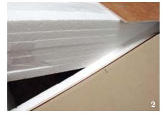
The cardboard box is lined on all sides, the top and bottom with 1/4-inch plywood, and is stacked full of 1-inch polystyrene sheets, making a very rigid package.
