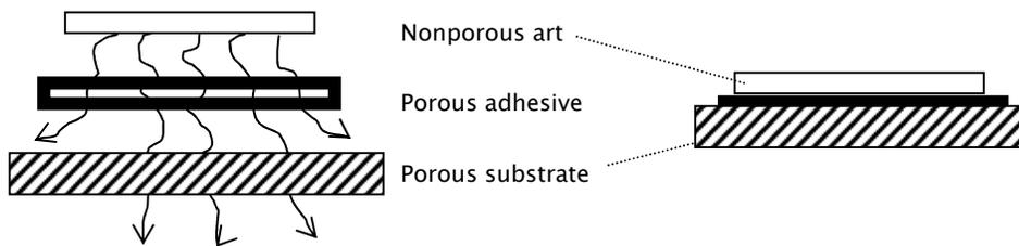
If a breathable item is to be mounted to a breathable substrate, essentially any tissue may be used to mount it simply because air will always be able to be compressed out through and around the porous art and substrate.
