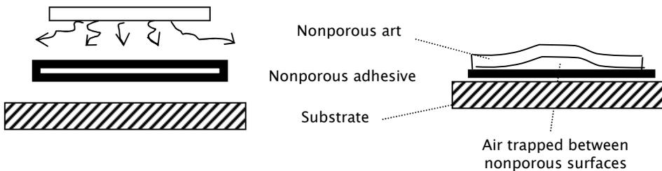
In any mounting or laminating package, only one layer within the sandwich between release materials on top and bottom may be nonporous. If two exist, such as photo and adhesive, or photo and nonperforated laminate, air is likely to remain trapped between the layers in the completed mounting. In other words, the project will suffocate. Only one layer in any mounting or laminating package may be nonporous, all others must be allowed to breathe.
