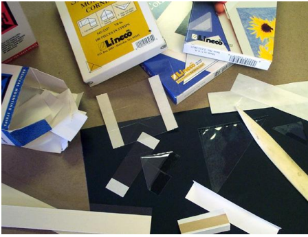
photo 1 Clockwise from upper left: ArtSaver Archival Mounting Strips; Lineco Archival Mounting Corners, Mylar Photo Corners, and Polypropylene Framers Corners; See-Thru polyester Mounting Strips and bone burnishers make up a few of the available pressure-sensitive edge strips and corner pockets.
