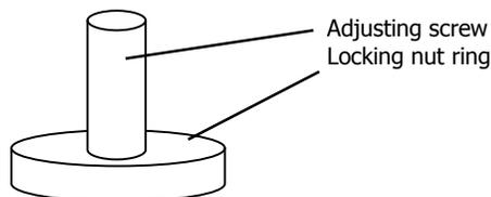
Twisting the adjusting screws evenly to the right or in a clockwise position will drop the lever arm down, thus lightening or decreasing the press pressure. Twisting the nuts to the left or counterclockwise will raise the arm up and increase the press pressure. It's best to turn both screws at the same time when adjusting.
