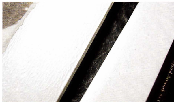
Adhesive (L) has a definite pattern while the coating (R) is smoother. Thin images can allow orange peel to show through after mounting if the adhesive does not flatten when melted.
