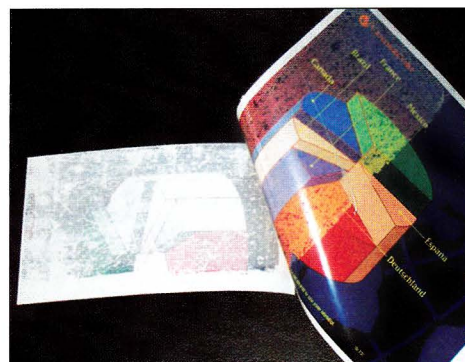
Photo 1: Thermal Transfer on Film—The digital image on right in this photo was printed using a Tektronix Phaser 240 thermal transfer system on film for overhead projector. The upper half of the film has melted and destroyed the image. The half sheet of single sided release paper to its left shows the ink residue that melted and transferred. This is a disaster that cannot be repaired.
