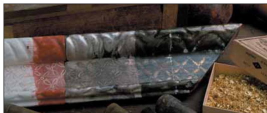
Gesso, bole, and moulding sample by Max Kuehne shows the developmental stages of the gilding process from raw wood, gesso (white), bole, (red), silver leaf with oxidized silver, and gamboge finish. Photo: Eddie Owen, Gold Leaf Studios, Washington, DC.
