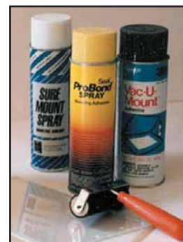
Typical spray mounting products from the past, with a rubber brayer for manual application.
