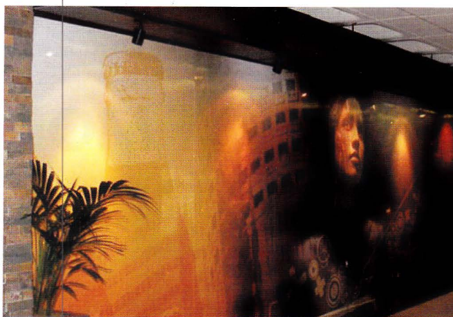
A decorative café wall installation was created on MDF by a solvent flatbed printer.
