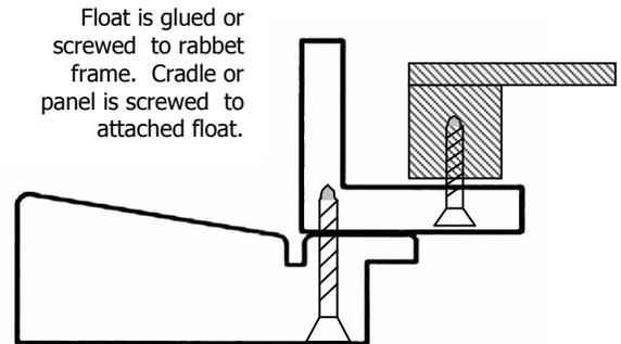
Float is glued or screwed to rabbet frame. Cradle or panel is screwed to attached float.
