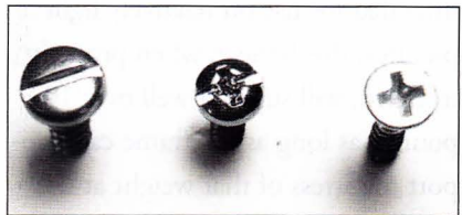
Slotted drive, pan head (L), Combination drive, pan head (C), and Phillips drive, flat head (R).
