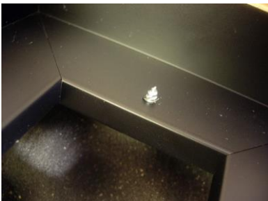
photo 14 - Install Screws Install the screws all the way through the frame so that 1/8" of the threading juts out the front
