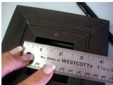
photo 9 - Marking for Screws The entry points were to be 1/4" in on all sides. Only one screw was needed each side because of the small size of the art.
