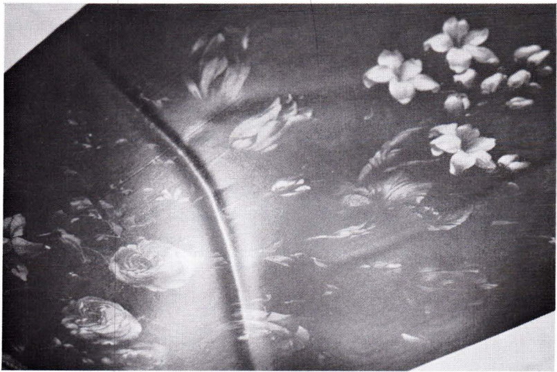
Photo 13: The hump created during the initial laminating stage of mounting is the result of no solid substrate or release board support when using a heat vacuum press. Wrinkles in the rubber bladder or felt can imprint into the art. This will disappear during the second canvas transfer mounting as long as a board is used beneath it.
