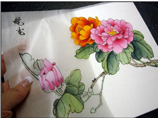
PHOTO 10 DRY MOUNTED SpeedMount was used for this sample, with only the right half of the silk having been mounted. It was bonded in a mechanical press of 155°F for 30 seconds and cooled under a weight.
