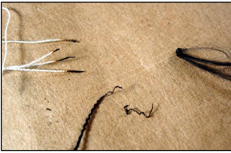
PHOTO 3 SILK FROM SYNTHETIC (L to R) Natural raw silk or silk blends will burn down the thread much like a candle wick leaving the burnt fiber. Linen burns down the thread but leaves a powdered ash where the thread was, and polyester silk will melt into a glob.
