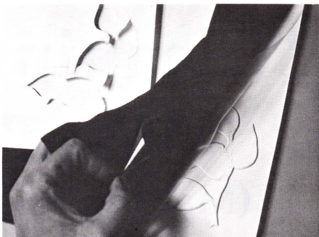
Photo 7A: From photo right to left: \frac{3}{16} " acid-free foam window mat (pattern ATG applied), Fusion 4000 pure film adhesive, velour fabric, pattern template (4ply board).
