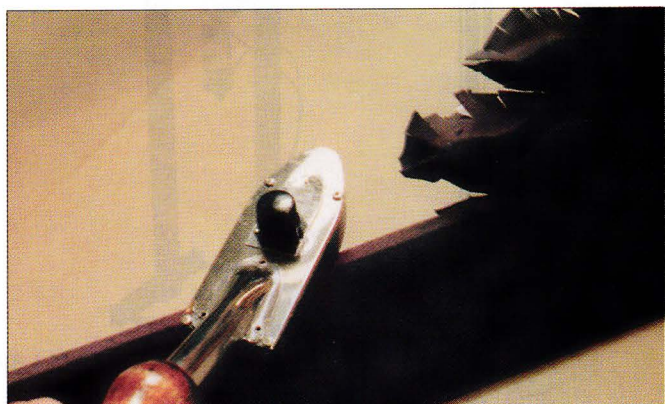
Photo 6: Iron the bevel to reactivate unmelted adhesive.
