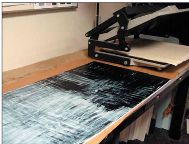
Wet glues may be brushed or applied with a roller. The glue here was brushed on a black rag board in preparation for the dry application of brown linen.
