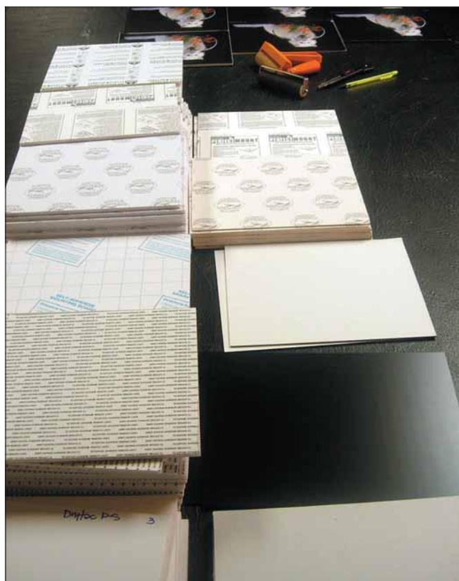
P-S adhesives come as pre-adhesived boards with a liner, as in this photo, or as films that can be used with your substrate of choice.
