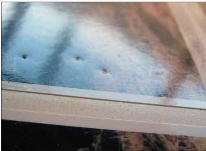
Routine cleaning of press platens and wiping of all release materials, prints, and substrate will prevent indentations caused dirt within the press.
