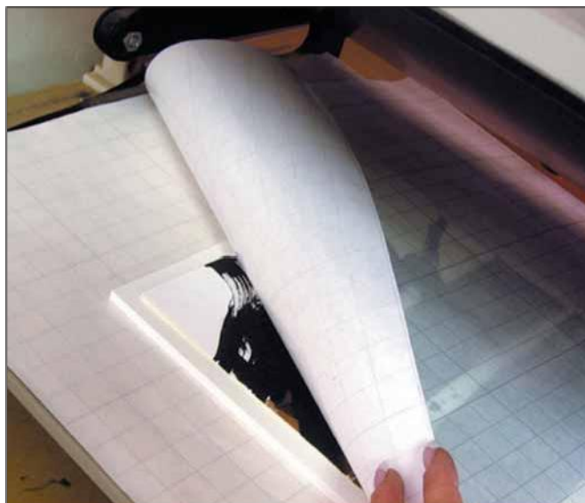
Print and adhesive are tacked to substrate and placed between release materials for bonding in a dry mount heat press.
