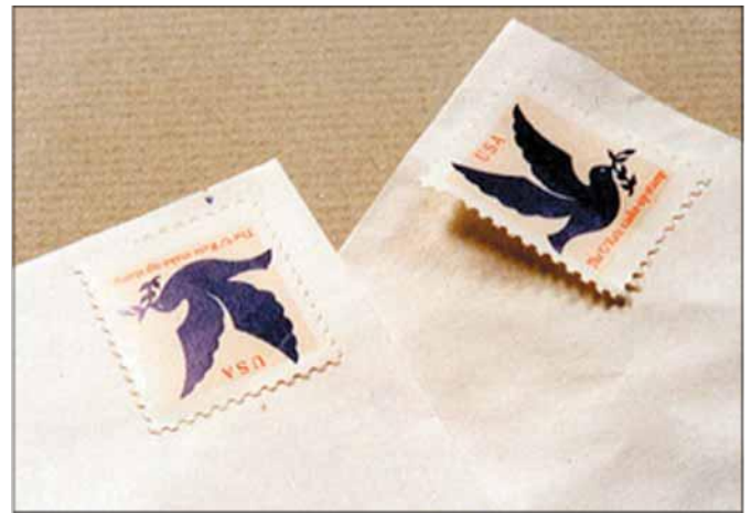
A lick 'n stick stamp will not stick to a wet envelope (right). All layers must be dry to bond (left).
