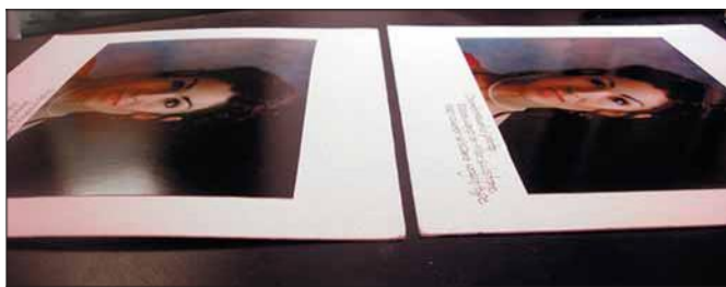
A traditional RC photo mounted to 2-ply rag (left) is warped. The same photo and 2-ply rag counter-mounted lies flat (right).
