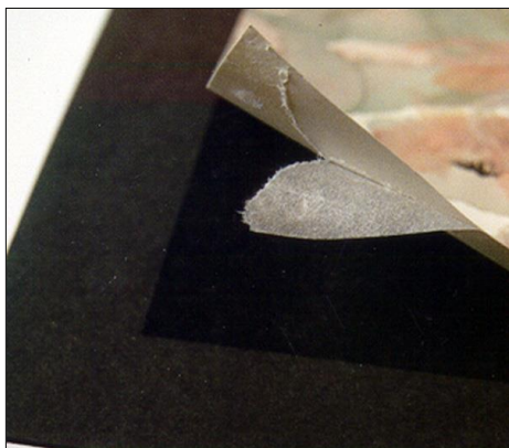
PHOTO 8 TOO HOT, TOO LONG
