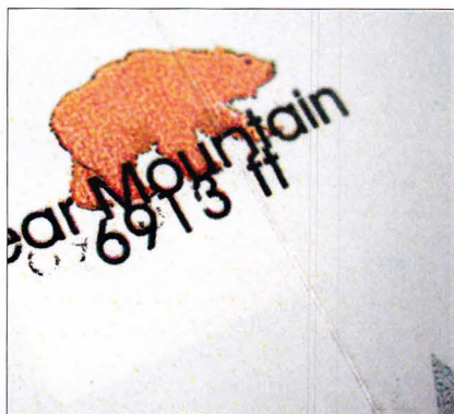
Photo 9: The ghosted arrow in the lower right corner and the reprint of the elevation numbers next to the name and numbers are a common problem when dry mounting laser prints.
