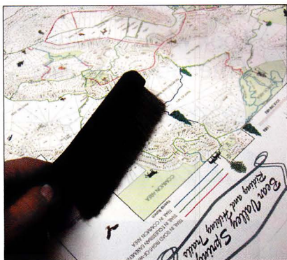
Photo 11: A Kinetronics anti-static brush helped remove all dust, particles, and dirt from the surface without creating additional static prior to covering with the laminate.
