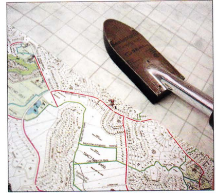
Photo 8: Clean Drytac single-sided release paper was used for this project, and the two halves of the map were aligned and tacked in place for the full length of the middle seam.
