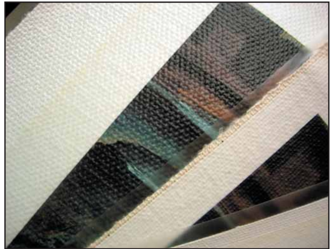
Photo 1: Photos in traditional transfers are surface laminated, peeled, and then aligned and mounted to a heat-activated canvas.
