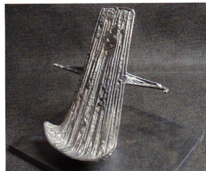
Steel rods were welded together and shaped to create a cradle that fit the back of the mask hollow.
