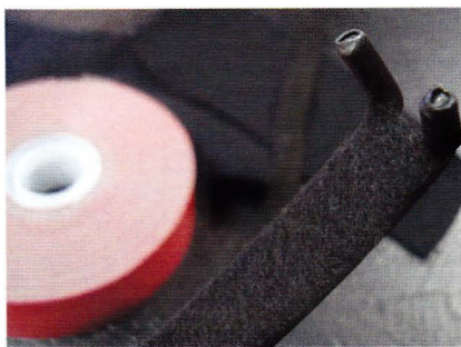
The end teeth are capped with shrink-to-fit plastic for additional padding and support.
