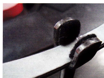
Each of the front metal flanges is backed with a felt pad. The flange pads are attached prior to aligning the felt in the curved support and after the liner has been removed.
