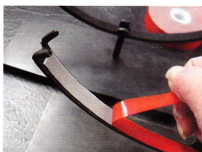
The plastic release liner is peeled off prior to adding flange felt.
