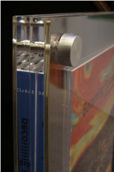
photo 9 Two 3/8" sink mats are fitted between clear 1/8" front and back sheets for the book in this enclosure.
