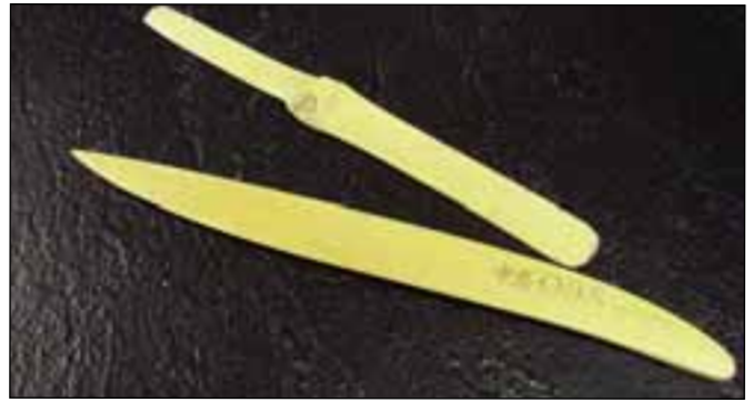
A homemade knife made from dried bamboo (top), and a commercial knife/burnisher (bottom)
