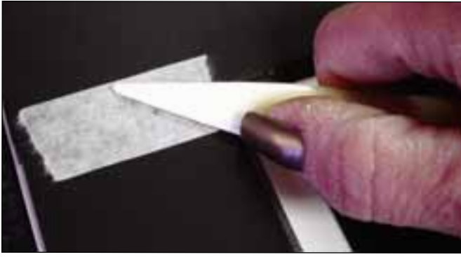
Spacer butt joints are reinforced with Lineco Abaca P-S tape and burnished.
