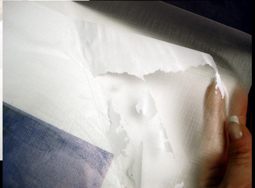
Digital press toner lifts ink from paper when laminate is lifted to realign
