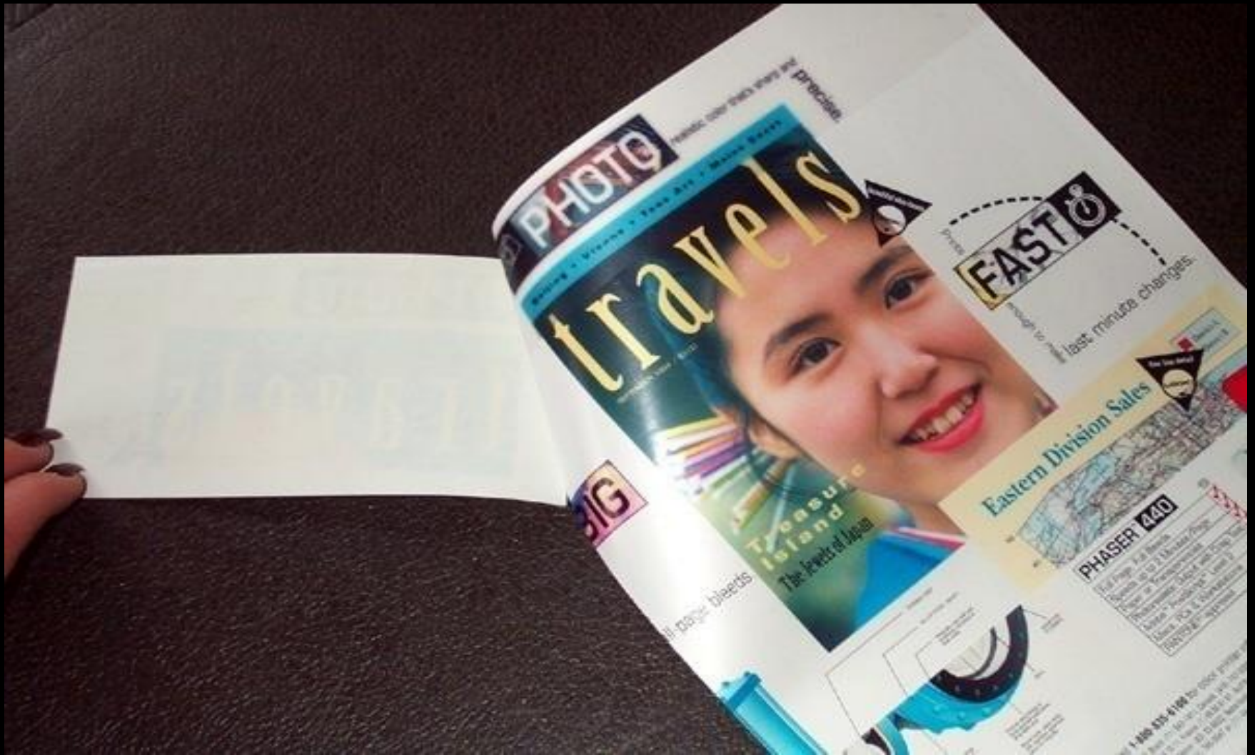
Solid Ink – Phase Change Inkjet Note faint image transfer on release paper
