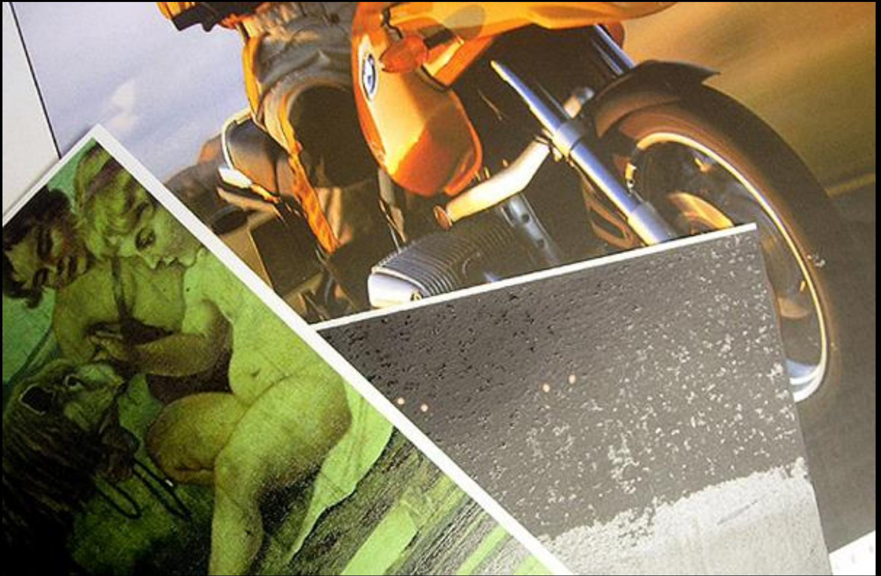
Electrophotographic four color toner copies and heat damage
